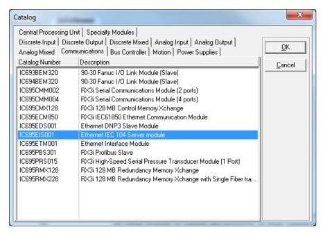
Once *added* to the rack location, set up the EIS001 parameters in the *Settings* and *RS-232 Port (Station Manager)* tabs as needed for the application.
